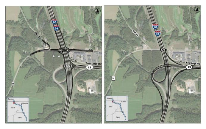
Figure 22: WIS 13 Interchange Split Diamond Design (WisDOT 2024c); Figure 23: WIS 13 Interchange Trumpet Design (WisDOT 2024c)
